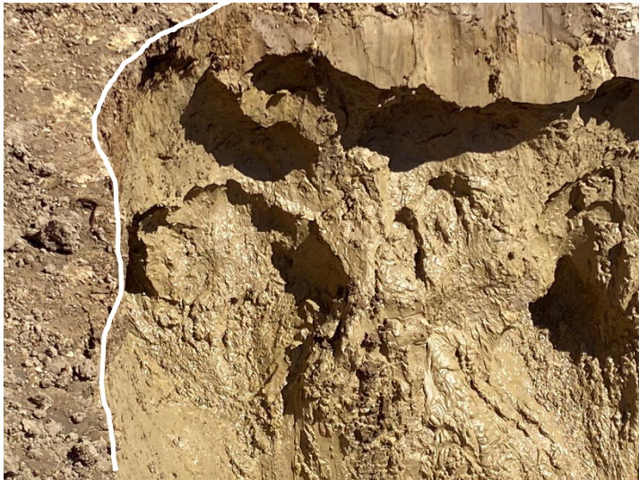
Photo 6: TP02-24 (May 3, 2024, after 24 hours of being excavated). Looking to the northwest. Note that soil sloughing of the test pit walls has occurred.
