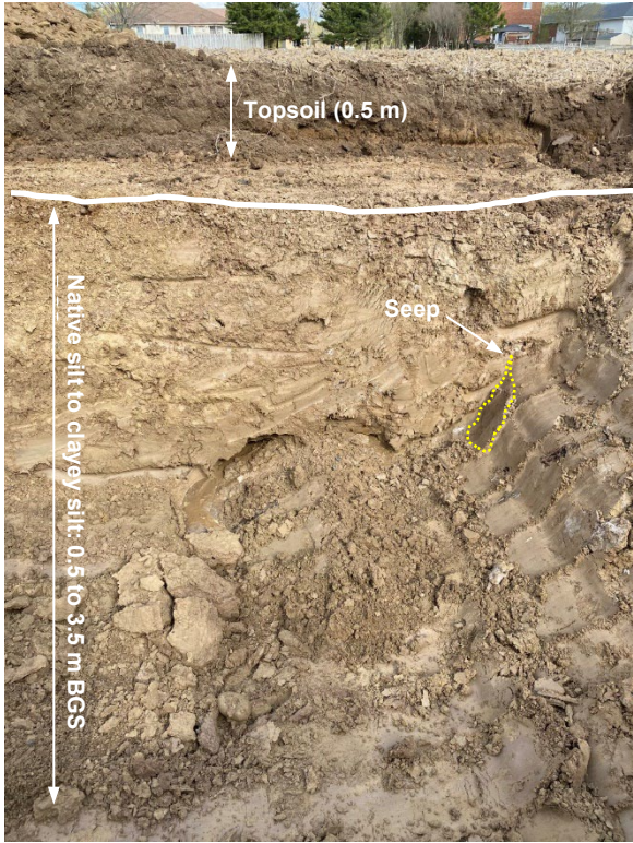
Photo 10: TP03-24 (May 2, 2024). Beginnings of seeping / flowing sand seam in southeast corner of the test pit.
