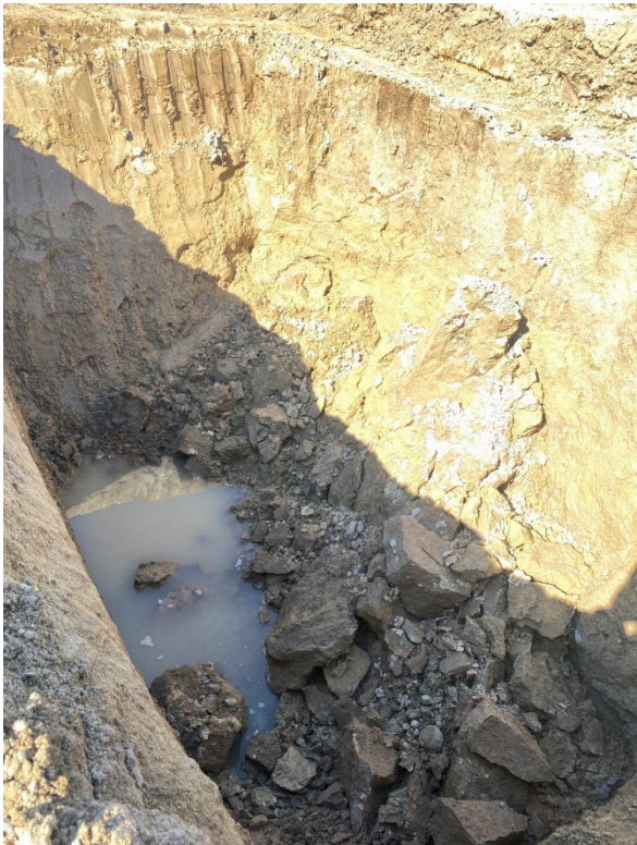
Photo 19: TP05-24 (May 3, 2024). Looking to the northeast. Note that soil sloughing of the test pit walls have occurred. Standing water is a byproduct of sand seam drainage.
