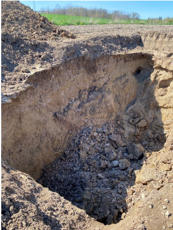
Photo 6: TP02-24 (May 3, 2024, after 24 hours of being excavated). Looking to the northwest. Note that soil sloughing of the test pit walls has occurred.
