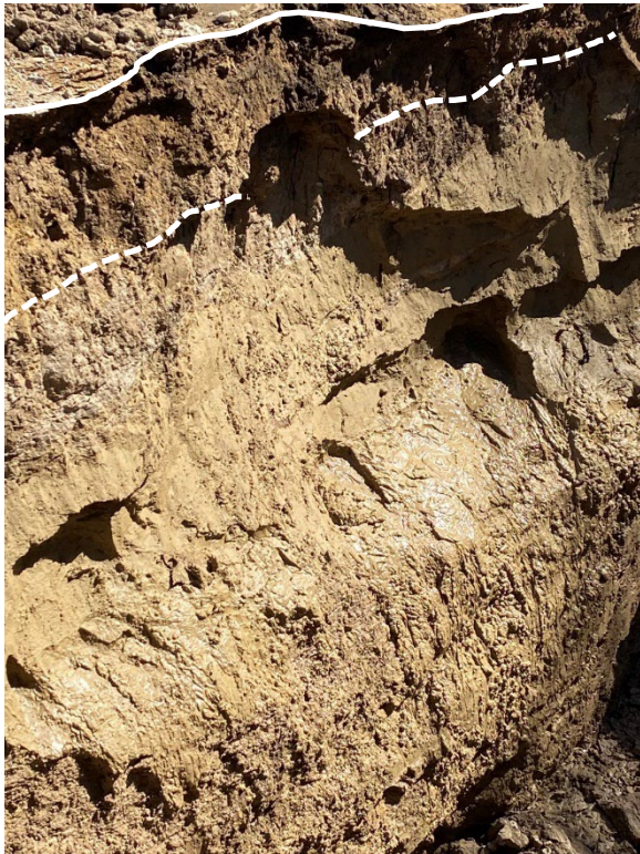
Photo 4: TP01-24 (May 3, 2024). Western face of test pit. From top of dashed white line to test pit bottom the wall is "sweating", an indication that groundwater is very slowly seeping from the wall.
