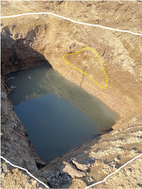
Photo 14: TP04-24 (May 3, 2024, after 24 hours of being excavated). Standing water is a byproduct of gravelly sand seam drainage.
