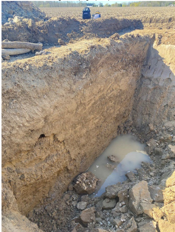
Photo 20: TP05-24 (May 3, 2024, after 24 hours of being excavated). Looking to the northwest. Note that seepage from sand seam had stopped (i.e., drained out).
