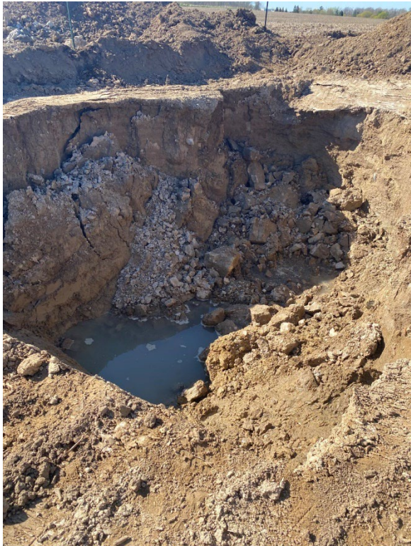
Photo 12: TP03-24 (May 3, 2024, after 24 hours of being excavated). Note that soil sloughing of the test pit walls have occurred. Standing water is a byproduct of sand seam drainage.
