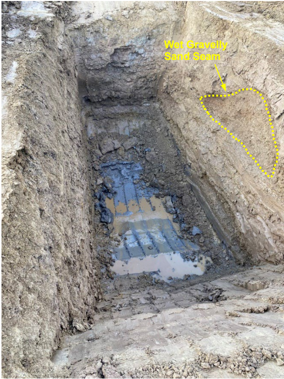
Photo 13: TP04-24 (May 2, 2024). Looking at east face of test pit. Observed draining of gravelly sand seam into test pit at time of excavation.
