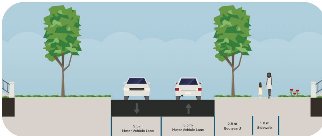
Figure 5: Sample Cross Section for a Neighbourhood Local Street, Sidewalk on One Side
