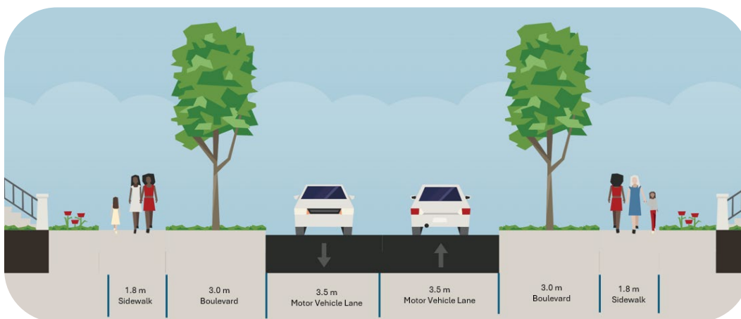
Figure 6: Sample Cross Section for a Neighbourhood Local Street, Sidewalks on Both Sides
