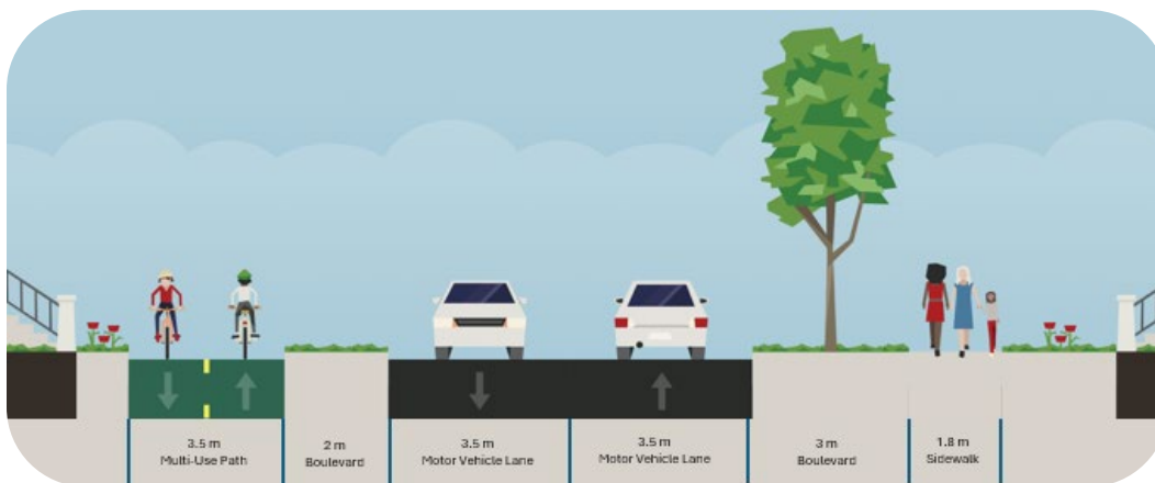
Figure 7: Sample Cross Section for a Neighbourhood Local Street with Multi-Use Path
