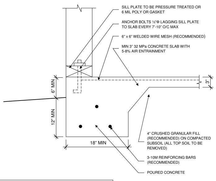
**NOTE:** THIS SLAB DESIGN IS FOR DETACHED GARAGES AND SHEDS. THE AREA MAY NOT EXCEED 55m<sup>2</sup> (592 ft<sup>2</sup>), MAXIMUM ONE STOREY IN BUILDING HEIGHT AND NO BRICK/MASONRY VENEER.
