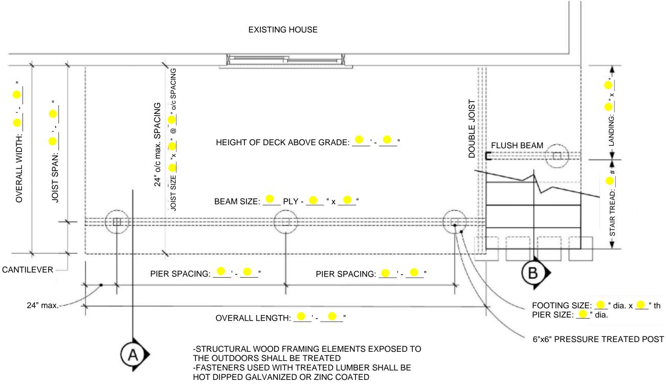
$\frac{\text{DECK FRAMING PLAN}}{\text{N.T.S.}}$
